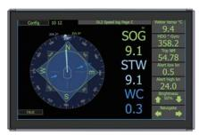
The SKIPPER DL1 Multi is a Single Axis Doppler Speed Log, working on the doppler principle, providing longitudinal ship's speed (STW) and distance relative to sea water.
